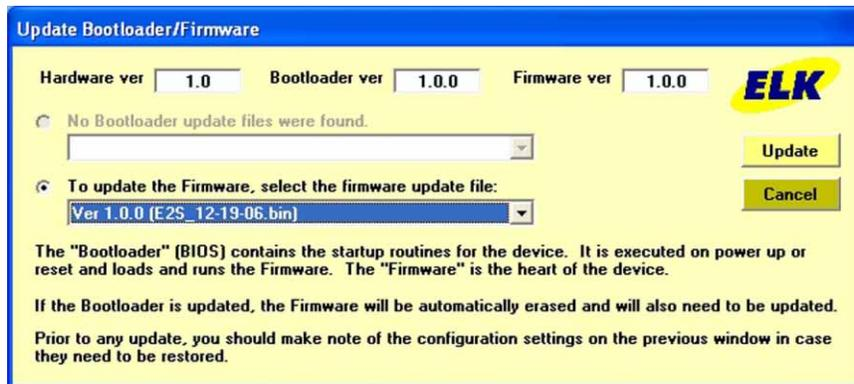
7. When the screen indicates that the update is complete, wait for the device to reboot. **DO NOT INTERRUPT OR POWER DOWN THE UNIT UNTIL THIS PROCESS IS COMPLETE!**
