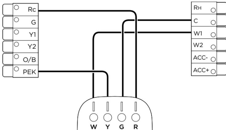
**NOTE** Do not connect any jumper wires between Rc and Rh. ecobee does this automatically. The R wire needs to go into the Rc terminal on your ecobee.
